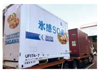
"Hyokan Soko" that manages a standard temperature via external power when stored and secondary battery power when in transport
